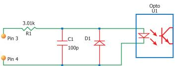
Figure B: Internal ON/OFF pin circuitry
