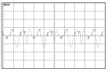
**Figure 10:** Output voltage ripple, Vout, at nominal input voltage and rated load current (50 mV/div). Load capacitance:  $1\mu F$  ceramic and 10mF tantalum capacitors. Bandwidth: 25 MHz. See Figure 17. Horizontal Scale:  $2\mu s/div$
