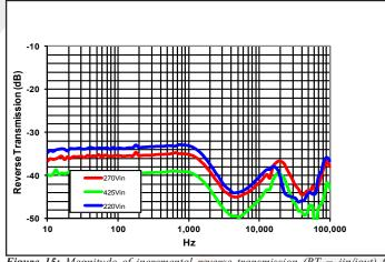
*Figure 15:* Magnitude of incremental reverse transmission (RT = iin/iout) for minimum, nominal, and maximum input voltage at full rated power. Cout=10mF
