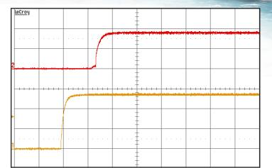
Figure 8: Turn-on transient at full resistive load and zero output capacitance initiated by Vin. ON/OFF Pin previously low, Cout=10mF. Ch 1: Vin (100V/div). Ch 2: Vout (2V/div). Horizontal Scale: 100ms/div
