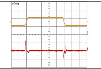
**Figure 12:** Output voltage response to step-change in input voltage  $(1V/\mu s)$ . Load cap: 10 mF electrolytic output capacitance. Ch 1: Vin (200V/div), Ch 2: Vout (50mV/div, enhanced resolution). Horizontal Scale:  $500\mu s/div$
