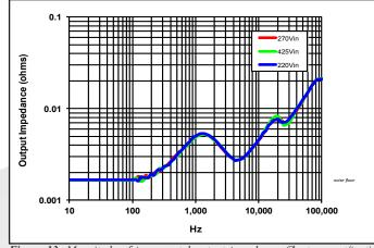
Figure 13: Magnitude of incremental output impedance (Zout = vout/iout) for minimum, nominal, and maximum input voltage at full rated power. Cout=10mF
