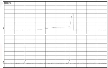
**Figure 18:** Load current (20A/div) as a function of time (0.5ms/div and 50ms/div) when the converter attempts to turn on into a 10 m $\Omega$  short circuit. Cout=10 $\mu$ F
