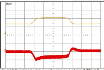
**Figure 11:** Output voltage response to step-change in load current (50%-75%-50% of lout(max);  $dI/dt = 0.1 A/\mu s$ ). Load cap:  $1 \mu F$  ceramic and 10mF tantalum capacitors. Ch A: lout (50A/div), Ch 2: Vout (200mV/div). Horizontal Scale: 500 $\mu s/div$
