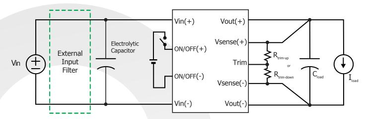
Figure D: Typical application circuit
