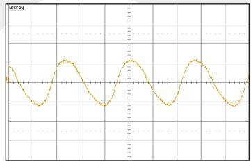
**Figure 9:** Input terminal current ripple,  $i_{c}$ , at full rated output current and nominal input voltage (200 mA/div), Cout=10mF. Bandwidth: 20MHz. See Figure 17. Horizontal Scale: 1µs/div
