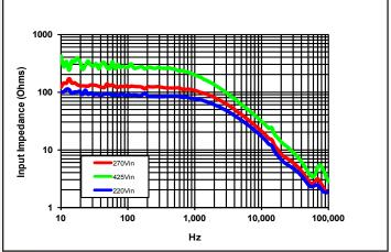
Figure 16: Magnitude of incremental input impedance (Zin = vin/iin) for minimum, nominal, and maximum input voltage at full rated power. Cout=10mF
