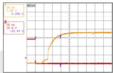
*Figure 7:* Typical startup waveform from Enable. Input voltage pre-applied, Cout=10mF. Ch 1: Vout (1V/div). Ch 2: Enable pin to Vin- (1V/div). Horizontal Scale: 20ms/div
